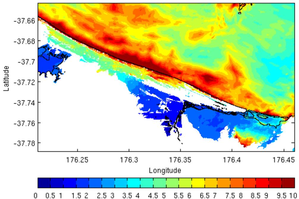
Figure 2.9 For the variation of the Whole Kermadec Scenario the detailed inundation modelling identifies the extent of inundation inland along the Papamoa and Te Tumu coastlines. The sand dunes between Te Tumu and the Kaituna River Mouth prevent the tsunami from inundating this part of the coastline. Most of the low-lying areas along the Maketu Estuary and Kaituna River Plain are inundated by the tsunami. Scale bar unit is in metres.
