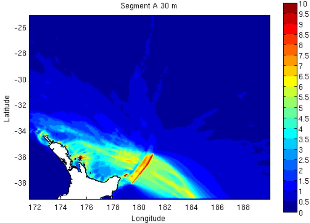
Figure A2.20 The maximum tsunami elevation above MHWS for the variation of the Southern Kermadec Scenario. This modelling shows a tsunami generated from the rupture mostly affects the east coast of the North Island, New Zealand. The colour scale shows the maximum tsunami elevation above MHWS. Scale bar unit is in metres.
