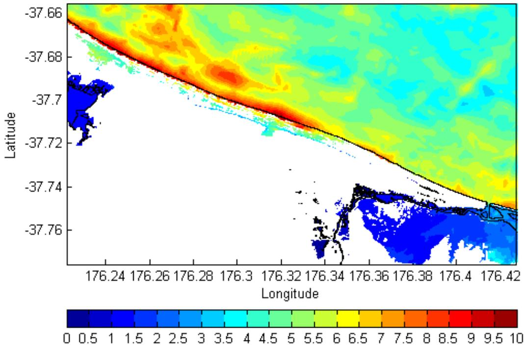
Figure 2.5 The maximum tsunami elevation above MHWS along the Papamoa and Te Tumu coastlines from the whole Kermadec scenario. No inundation occurs along the Te Tumu coastline as the sand dunes are high enough to prevent overtopping by the tsunami. The colour scale shows the maximum tsunami elevation above MHWS. Scale bar unit is in metres.
