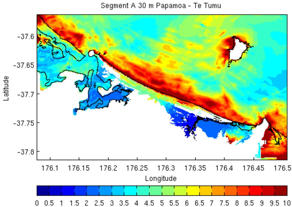
Figure 2.7 For the variation of the Southern Kermadec Scenario, the sub-regional model shows the maximum tsunami elevation varies between 8.0m and 15.0m above MHWS between the Maketu Estuary and Matakana Island. Significant inundation occurs at Papamoa and the north western half of the Te Tumu coastline. The colour scale shows the maximum tsunami elevation above MHWS. Scale bar unit is in metres.
