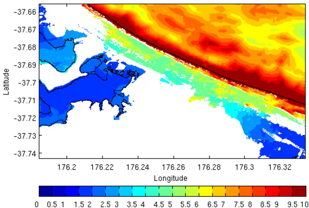
Figure A2.29 The maximum tsunami elevation above MHWS for the variation of the whole Kermadec Scenario. The inundation extends inland at Papamoia indicating that the tsunami has overtopped the sand dunes along the beach. The tsunami overland flows propagate further down to the low-lying areas towards Te Tumu. The colour scale shows the maximum tsunami elevation above MHWS. Scale bar unit is in metres.
