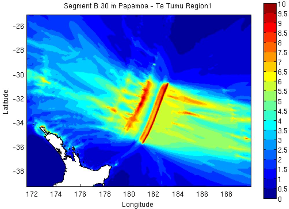
Figure A2.23 The maximum tsunami elevation above MHWS for the variation of the Central Kermadec Scenario. This modelling identifies that a tsunami generated from mostly affects the northern part of the East Coast of the North Island New Zealand. The colour scale shows the maximum tsunami elevation above MHWS. Scale bar unit is in metres.
