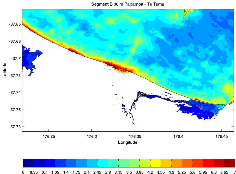
Figure A2.25 The maximum tsunami elevation above MHWS for the variation of the Central Kermadec Scenario. The detailed inundation modelling identifies localised inundation occurring along the Papamoa and Te Tumu coastlines. The tsunami from this event scenario is not capable of overtopping most of the sand dunes at Te Tumu. Localised inundation occurs at the low-lying area behind the Maketu Estuary. Scale bar unit is in metres.
