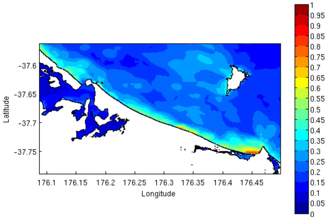
Figure A3.2 The maximum tsunami elevation for the Astrolabe Fault varies from 0.5m to 1.0m above MHWS along the east coast of the Bay of Plenty. The colour scale shows the maximum tsunami elevation above MHWS. Scale bar unit is in metres.
