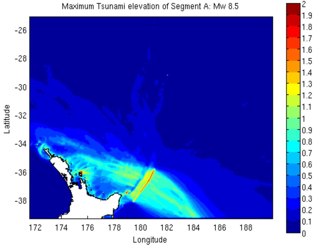
Figure A2.2 The maximum tsunami elevation above MHWS from the Southern Kermadec Scenario. The colour scale shows the maximum tsunami elevation above MHWS. Scale bar unit is in metres.
