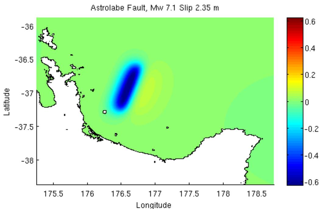
Figure A3.1 The initial condition of the tsunami elevation above MHWS from the Astrolabe Fault at the source region. The colour scale shows the maximum tsunami elevation above MHWS. Scale bar unit is in metres.
