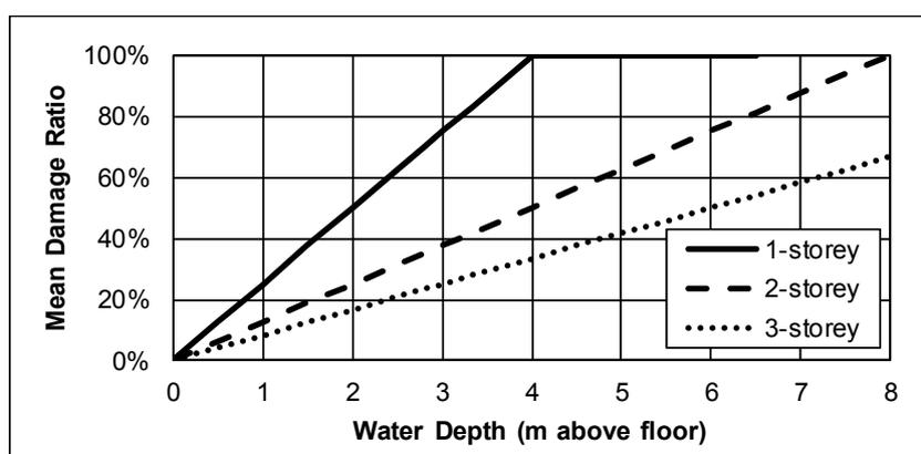
Figure 3.3 Tsunami fragility functions for concrete buildings.
