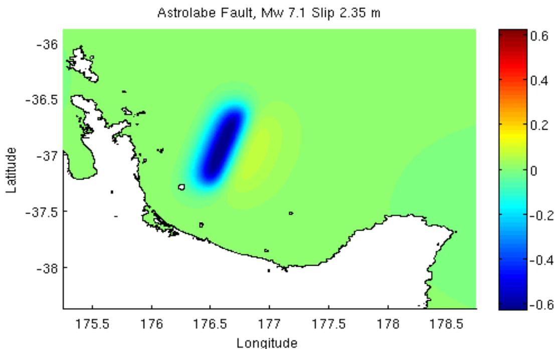
Figure 2.13 The initial sea surface displacements for the Astrolabe Fault scenario. Scale bar unit is in metres.
