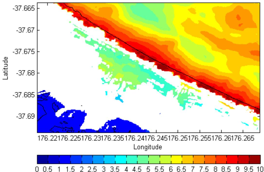
Figure A2.14 The maximum tsunami elevation above MHWS resulting from the whole Kermadec scenario for the Papamoa coastline nearer Mt Maunganui. In this area, the tsunami overtops the sand dunes and inundates the area behind. Scale bar unit is in metres.
