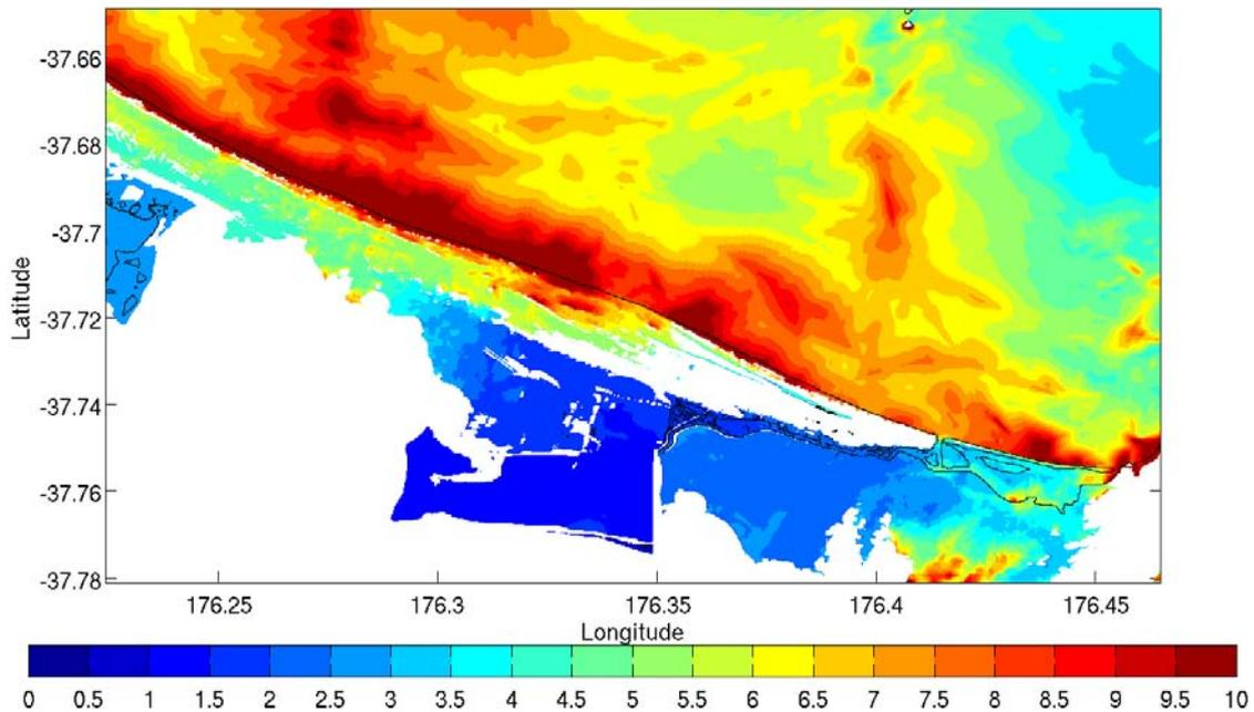
Figure A2.18 The maximum tsunami elevation above MHWS involving the Kermadec – Hikurangi Scenario along the Papamoa Coast near Mt Maunganui which shows extensive inundation occurring between Papamoa and Te Tumu. Scale bar unit is in metres.
