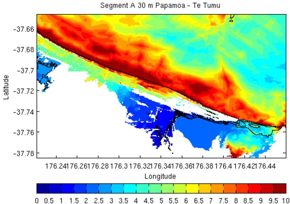
Figure A2.22 The maximum tsunami elevation above MHWS for the variation of the Southern Kermadec Scenario. Detailed inundation modelling shows the extent of inundation inland along the Papamoa and Te Tumu coastline. The ~12m high sand dunes along the coastline of Te Tumu towards the Kaituna River Mouth prevent the tsunami inundating this part of the region. Most of the low-lying areas along the Maketu Estuary and Kaituna River Plain are inundated by the tsunami. Scale bar unit is in metres.
