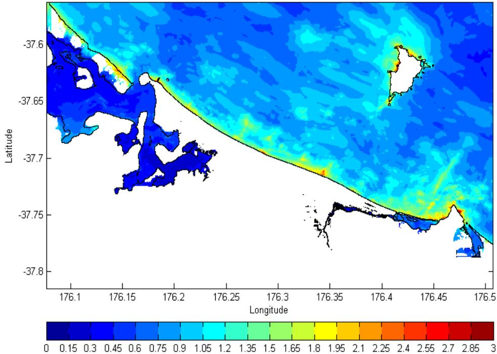
Figure A2.6 The maximum tsunami elevation above MHWS for the Central Kermadec Scenario for the coastline between Maketu Estuary and Matakana Island. The colour scale shows the maximum tsunami elevation above MHWS. Scale bar unit is in metres.
