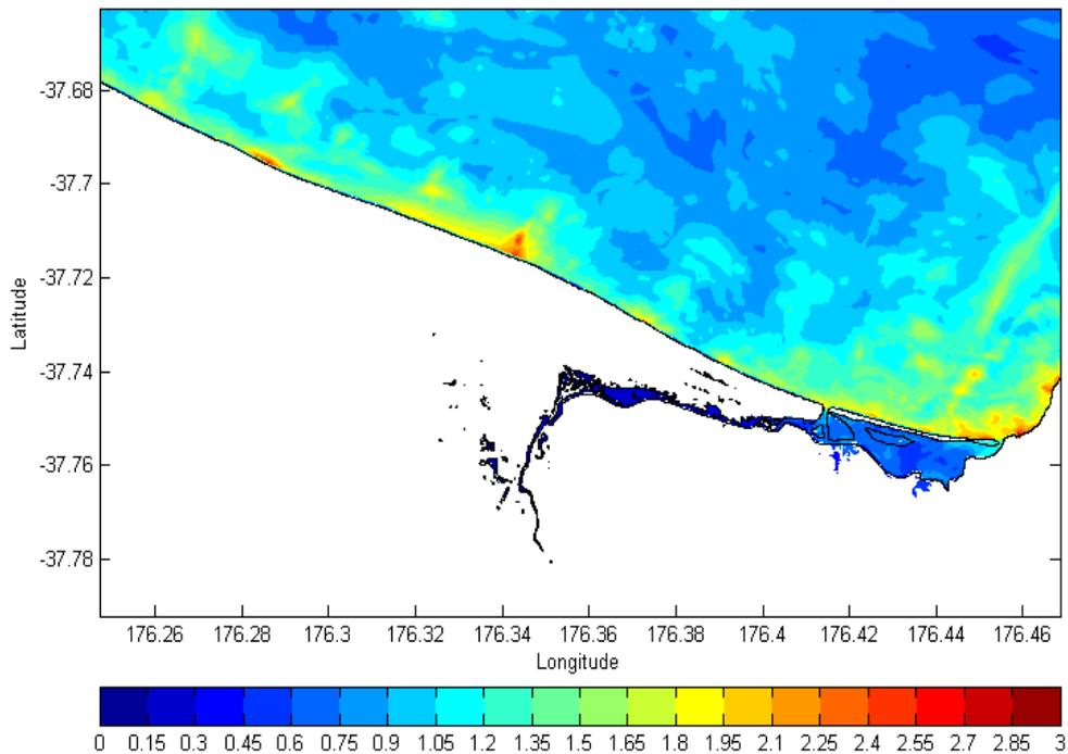
Figure A2.7 The maximum tsunami elevation above MHWS from the Central Kermadec Scenario for the Papamoia and Te Tumu coastlines. This modelling shows that there is no significant inundation except to the area around the Maketu Estuary. The colour scale shows the maximum tsunami elevation above MHWS. Scale bar unit is in metres.
