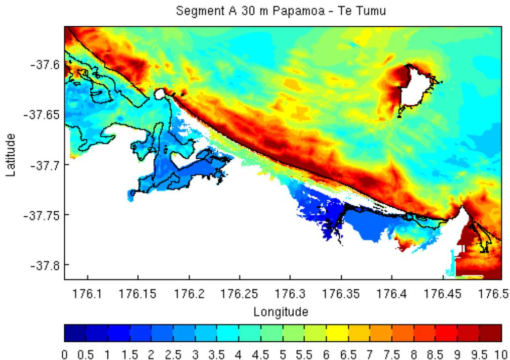
Figure A2.21 The maximum tsunami elevation above MHWS for the variation of the Southern Kermadec Scenario. The sub-regional model shows the maximum tsunami elevation varies between 8.0m and 15.0m above MHWS between Maketu Estuary and Matakana Island. Significant inundation occurs at Papamoa and the north western half of the Te Tumu coastline. Scale bar unit is in metres.
