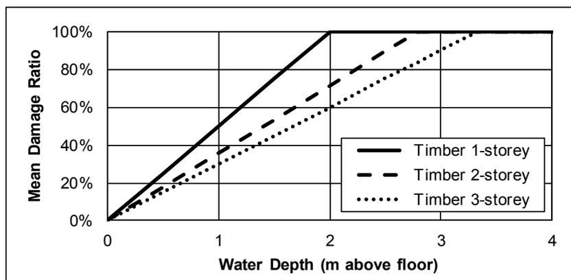
Figure 3.2 Tsunami fragility functions for timber buildings.
