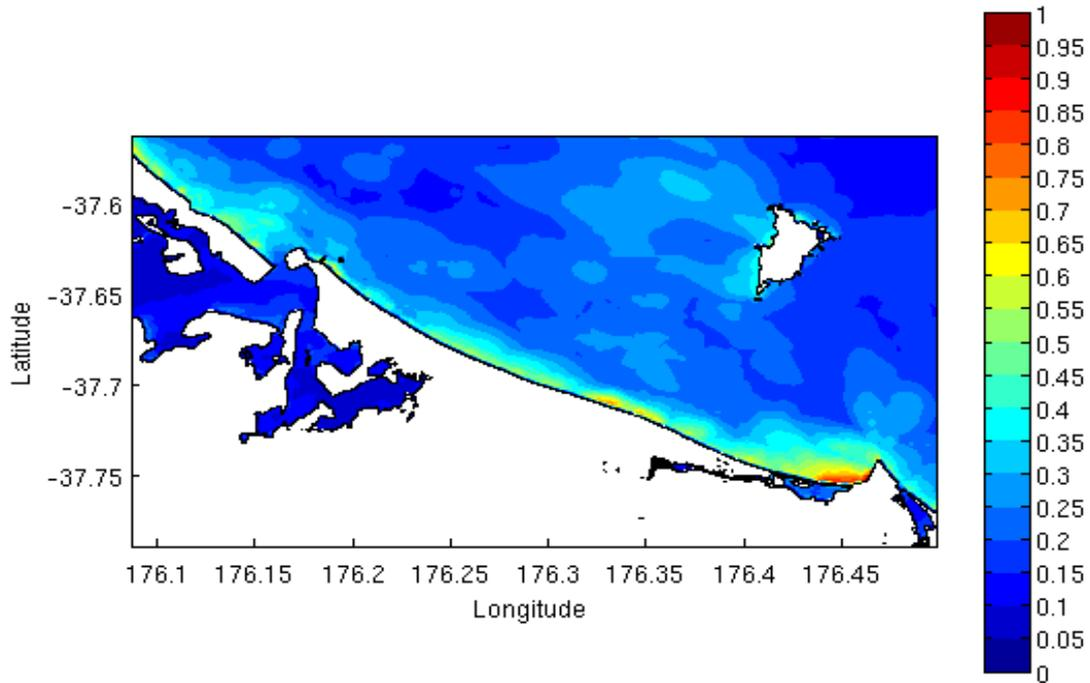
Figure 2.14 For the Astrolabe Fault Scenario, the maximum tsunami elevation varies from 0.5m – 1.0m above MHWS along the east coast of the Bay of Plenty. The colour scale shows the maximum tsunami elevation above MHWS. Scale bar unit is in metres.
