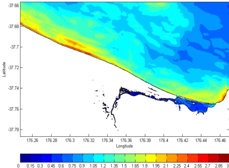
Figure A2.4 The maximum tsunami elevation above MHWS from the Southern Kermadec Scenario for the Papamoia and Te Tumu coastline. This modelling shows that there is no significant inundation except to the area around the Maketu Estuary. Scale bar unit is in metres.
