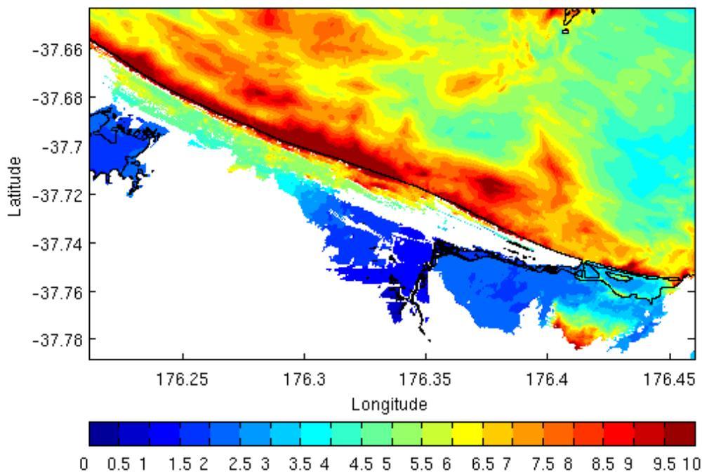
Figure A2.27 The maximum tsunami elevation above MHWS for the variation of the whole Kermadec Scenario. The sub-regional model shows the maximum tsunami elevation above MHWS varies between 8.0m – 15m between the Maketu Estuary and Matakana Island. Large scale inundation occurs at Papamoa and the north western portion of Te Tumu. The colour scale shows the maximum tsunami elevation above MHWS. Scale bar unit is in metres.
