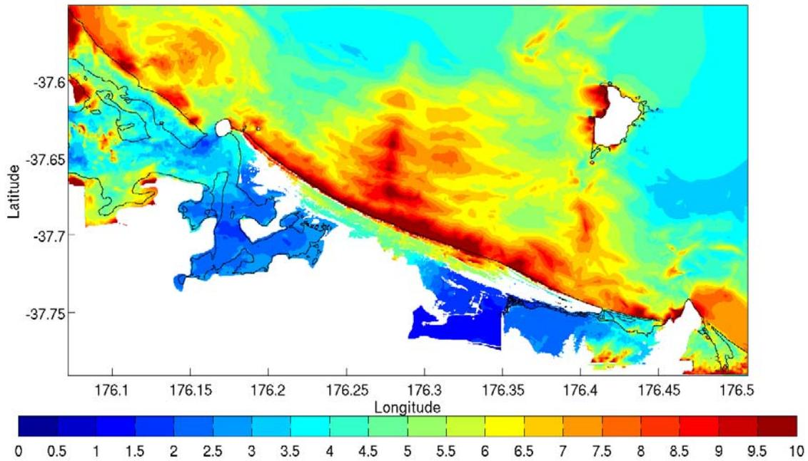
Figure A2.17 The maximum tsunami elevation above MHWS for the Kermadec – Hikurangi Scenario varies between 5.5m and 15.0m above MHWS between the Maketu Estuary and Matakana Island. Inundation occurs at several places along the coastline which includes Papamoa, Mt Maunganui and Matakana Island. Scale bar unit is in metres.
