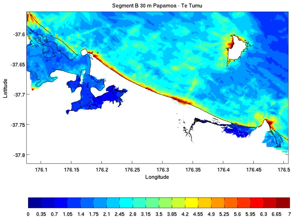
Figure A2.24 The maximum tsunami elevation above MHWS for the variation of the Central Kermadec Scenario. The sub-regional model shows the maximum tsunami elevation above MHWS varies from 3.0m – 8.0m above MHWS between the Maketu Estuary and Matakana Island. Scale bar unit is in metres.
