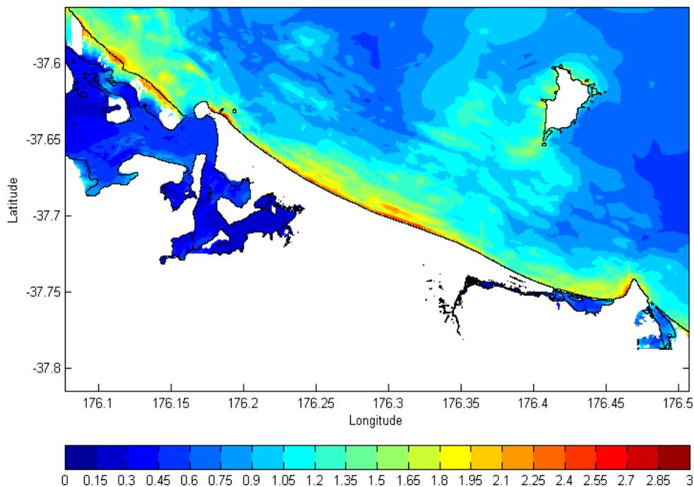
Figure A2.3 The maximum tsunami elevation above MHWS for the Southern Kermadec Scenario for the coastline between the Maketu Estuary and Matakana Island. The colour scale shows the maximum tsunami elevation above MHWS if it is offshore or flow depth if it is on land. Scale bar unit is in metres.
