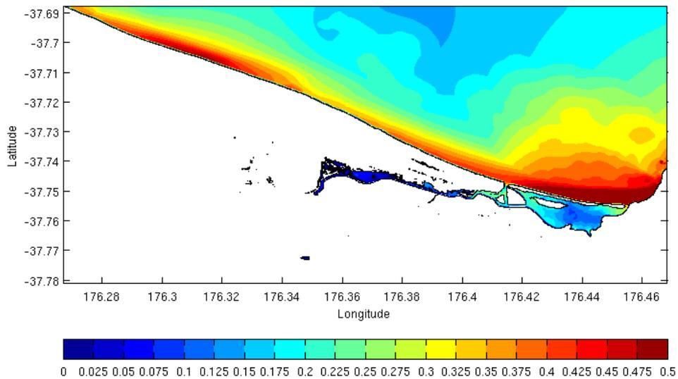
Figure A3.9 The maximum tsunami elevation varies between 0.2m and 0.7m above MHWS for the Composite White Island Fault along the Papamoa and Te Tumu coastlines. The colour scale shows the maximum tsunami elevation above MHWS. Scale bar unit is in metres.
