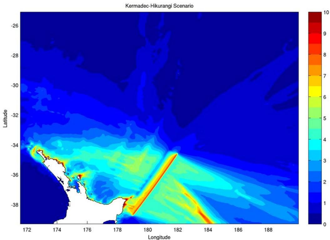
Figure A2.16 The maximum tsunami elevation above MHWS for the Kermadec – Hikurangi Scenario. This scenario shows most of the tsunami impact to the east coast of New Zealand originates from southern and central portions of the Kermadec Trench. East Cape is however significantly impacted as a result of the tsunami generated from the rupture of the northern portion of the Hikurangi Margin. The colour scale shows the maximum tsunami elevation above MHWS. Scale bar unit is in metres.
