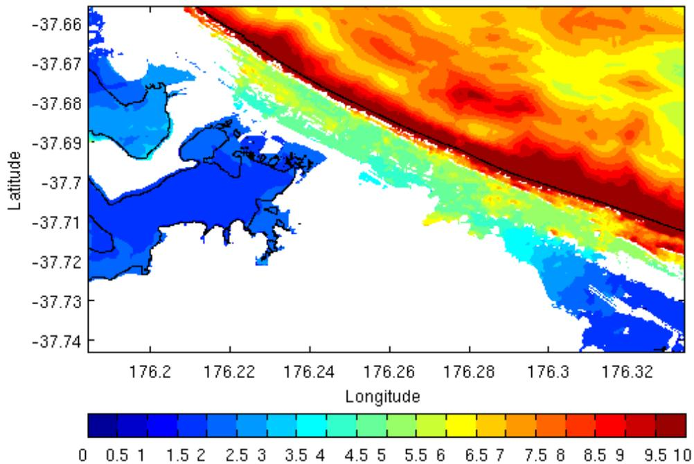
Figure 2.10 For the variation of the Whole Kermadec Scenario, the inundation extends inland at Papamoa indicating that the tsunami has overtopped the sand dunes along the beach. The tsunami overland flows propagate further down to the low-lying areas towards Te Tumu. The colour scale shows the maximum tsunami elevation above MHWS. Scale bar unit is in metres.
