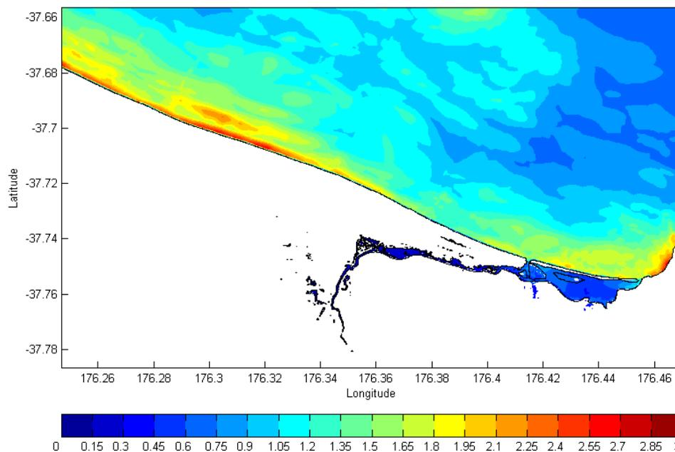
Figure 2.4 The maximum tsunami elevation above MHWS for the Southern Kermadec Scenario for the Papamoa and Te Tumu coastline. This modelling shows that there is no significant inundation except to the area around the Maketu Estuary. The colour scale shows the maximum tsunami elevation above MHWS. Scale bar unit is in metres.
