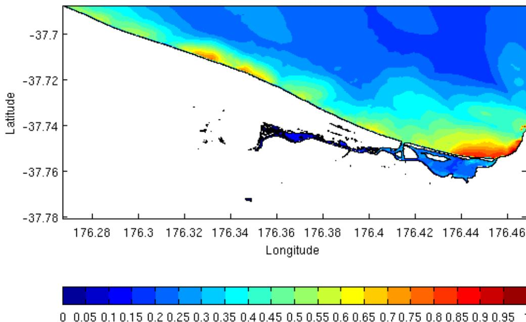
Figure A3.3 The maximum tsunami elevation varies from 0.2m – 0.6m above MHWS for the Astrolabe Fault along the Papamoa – Te Tumu coastline. At the Maketu Estuary the inundation may be up to 1.0m deep. The colour scale shows the maximum tsunami elevation above MHWS. Scale bar unit is in metres.
