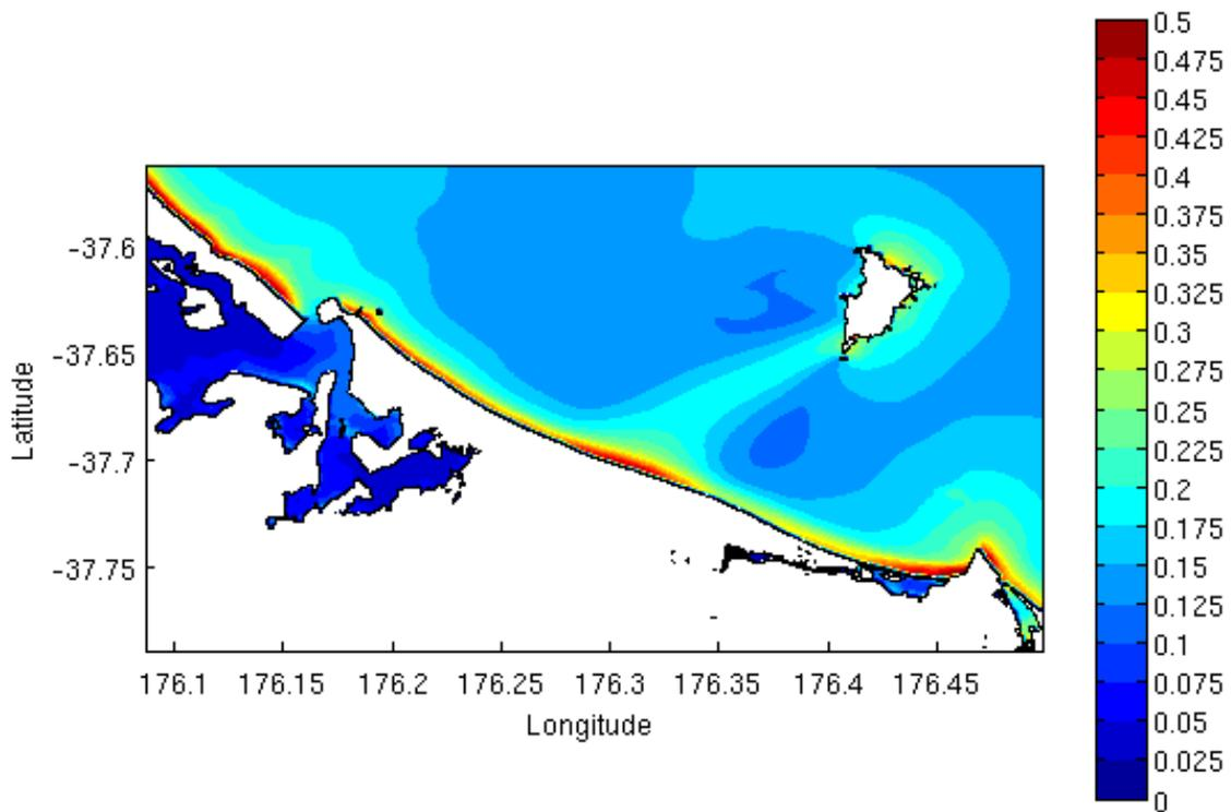
Figure A3.5 The maximum tsunami elevation varies from 0.3m to 0.7m above MHWS for the Volkner Fault along the Bay of Plenty coastline between the Maketu Estuary and Matakana Island. The colour scale shows the maximum tsunami elevation above MHWS. Scale bar unit is in metres.
