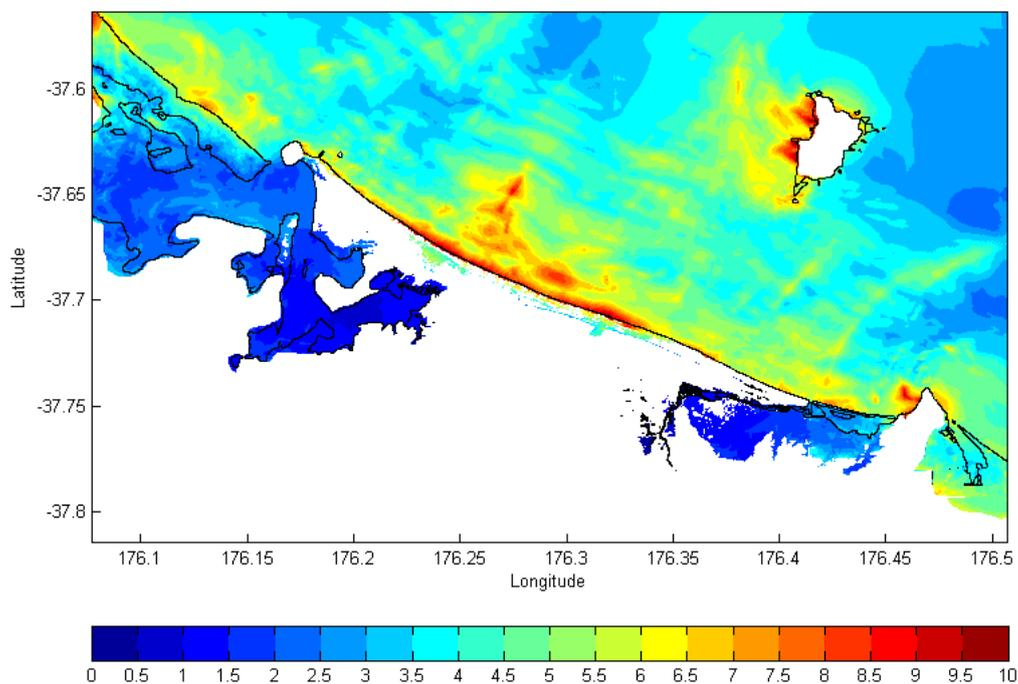
Figure A2.12 The maximum tsunami elevation above MHWS resulting from the whole Kermadec scenario. This modelling shows the maximum tsunami elevation varies from 5.0m – 10m above MHWS for the Bay of Plenty from the Maketu Estuary to Matakana Island. Inundation occurs at some places along the coastline such as Papamoa, Mt Maunganui and Matakana Island. Scale bar unit is in metres.
