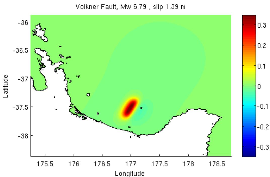
Figure A3.4 The initial condition of the tsunami elevation above MHWS for the Volkner Fault at the source region. The colour scale shows the maximum tsunami elevation above MHWS. Scale bar unit is in metres.
