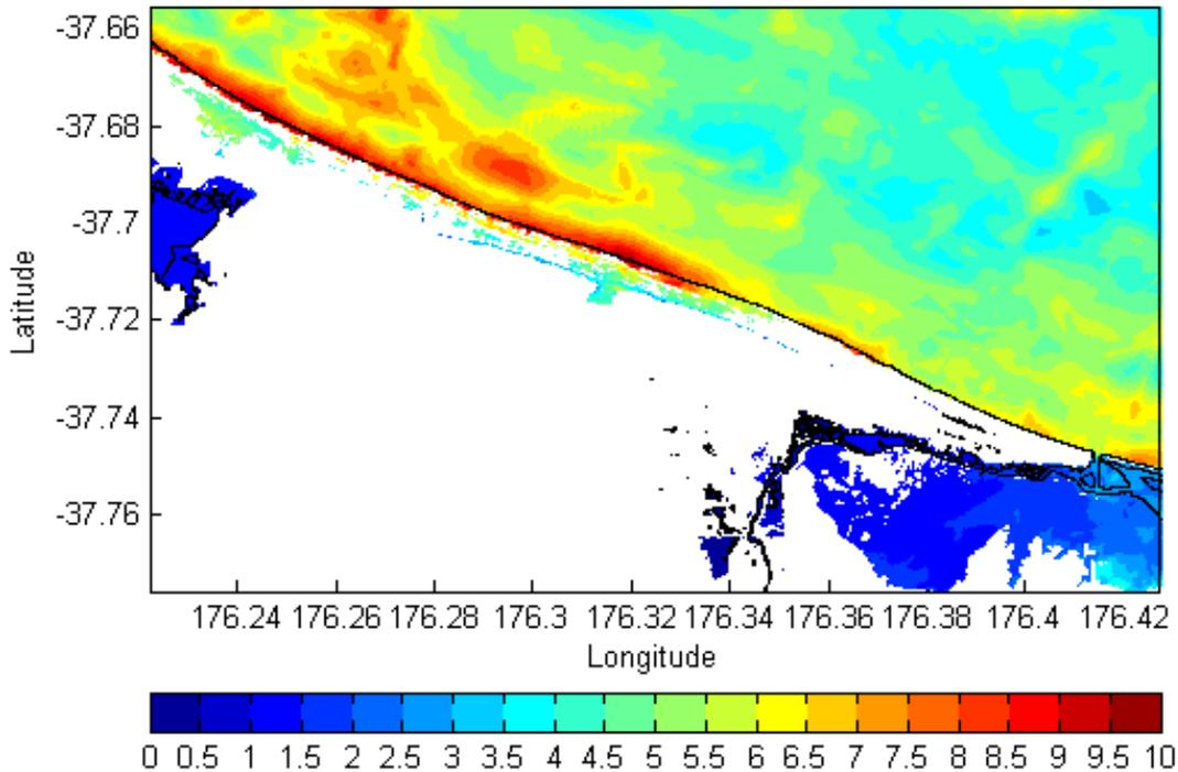
Figure A2.13 The maximum tsunami elevation above MHWS resulting from the the whole Kermadec scenario along the Papamoa and Te Tumu coastlines. No inundation occurs along the Te Tumu coastline as the sand dunes are high enough to prevent overtopping by the tsunami. Scale bar unit is in metres.
