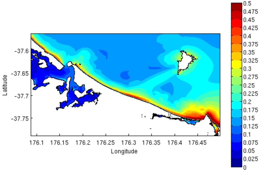
Figure A3.8 The maximum tsunami elevation varies between 0.2m and 0.7m above MHWS for the Composite White Island Fault along the Bay of Plenty coastline between the Maketu Estuary and Matakana Island. The colour scale shows the maximum tsunami elevation above MHWS. Scale bar unit is in metres.
