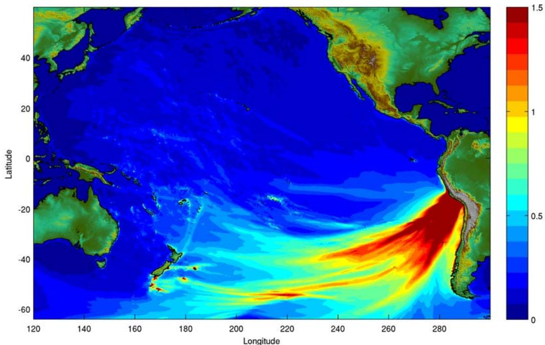
Figure 2.1 Maximum tsunami amplitude distribution for the Peru ( $M_w$  9.1) fault rupture, showing the tsunami directivity towards New Zealand. Scale bar unit is in metres.
