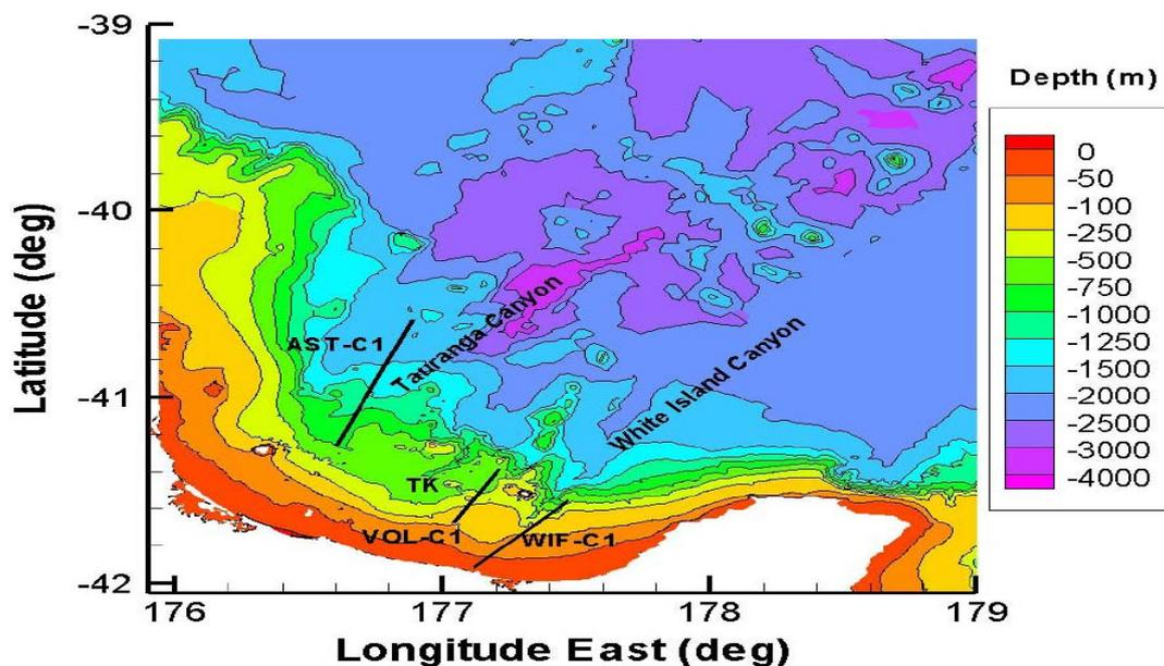
Figure 2.12 Fault delineation based on Lamarche and Barnes (2005) for the offshore environment of the Bay of Plenty (Walter et al. 2006). These have been used to assess the potential tsunami impact to the Papamoa – Te Tumu suburbs.
