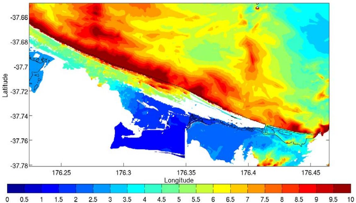
Figure 2.6 Detailed inundation pattern along Papamoa coast near Mt Maunganui which shows extensive inundation occurring between Papamoa and Te Tumu from the Kermadec - Hikurangi Scenario. The colour scale shows the maximum tsunami elevation above MHWS. Scale bar unit is in metres.
