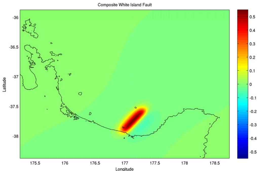
Figure A3.7 The initial condition of the tsunami elevation above MHWS for the Composite White Island Fault at the source region. The colour scale shows the maximum tsunami elevation above MHWS. Scale bar unit is in metres.
