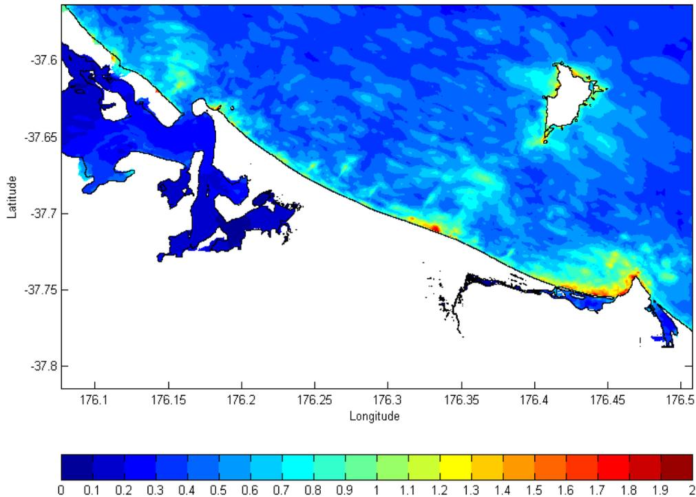
Figure A2.9 The maximum tsunami elevation above MHWS from the Northern Kermadec Scenario for the area between Maketu Estuary and Matakana Island. The colour scale shows the maximum tsunami elevation above MHWS. Scale bar unit is in metres.
