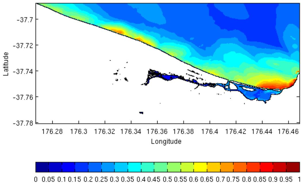
Figure 2.15 For the Astrolabe Fault Scenario, the maximum tsunami elevation varies from 0.2m – 0.6m above MHWS along the Papamoa – Te Tumu coastline. At the entrance to the Maketu Estuary the inundation may be up to 1.0m deep. The colour scale shows the maximum tsunami elevation above MHWS. Scale bar unit is in metres.
