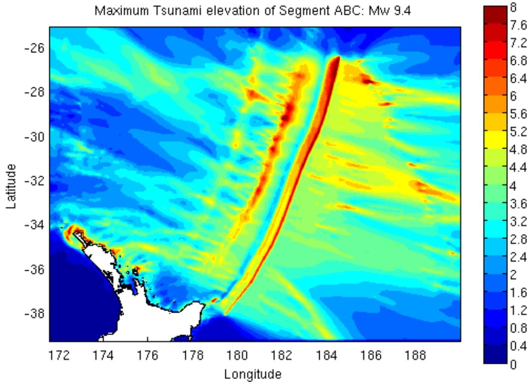
Figure A2.11 The maximum tsunami elevation above MHWS resulting from the whole Kermadec scenario. This modelling shows that the main source of the tsunami to impact the east coast of New Zealand is from the southern and central portions of the trench. The colour scale shows the maximum tsunami elevation above MHWS. Scale bar unit is in metres.
