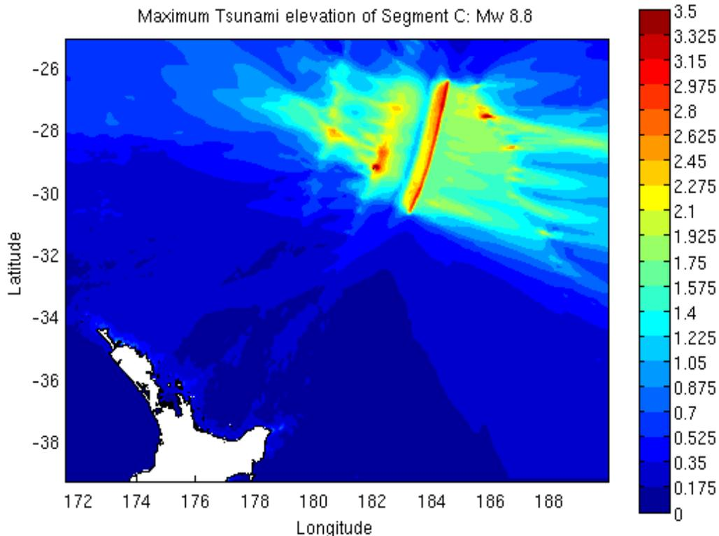
Figure A2.8 The maximum tsunami elevation above MHWS from the Northern Kermadec Scenario. A rupture would direct most of tsunami energy away from New Zealand. The colour scale shows the maximum tsunami elevation above MHWS. Scale bar unit is in metres.
