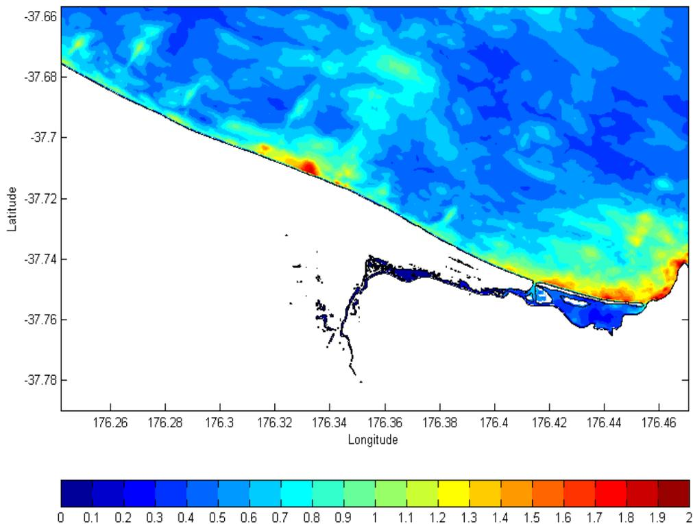
Figure A2.10 The maximum tsunami elevation above MHWS from the Northern Kermadec Scenario for the Papamoa and Te Tumu coastlines. This modelling shows that there is no significant inundation except to the area around the Maketu Estuary. The colour scale shows the maximum tsunami elevation above MHWS. Scale bar unit is in metres.
