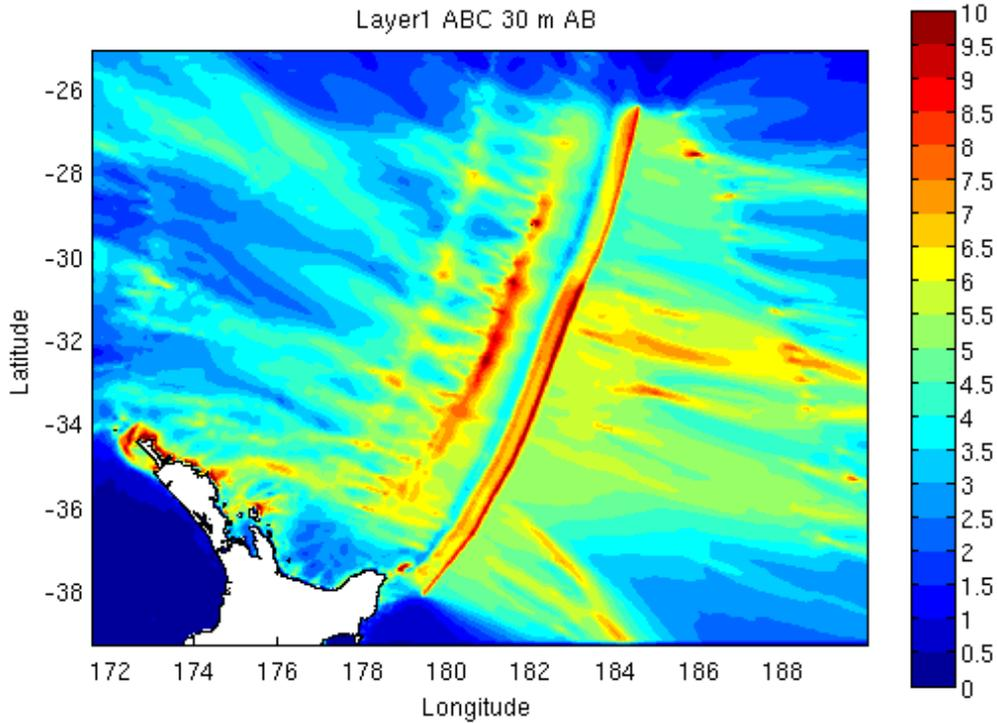
Figure A2.26 The maximum tsunami elevation above MHWS for the variation of the whole Kermadec Scenario. The modelling identifies that a tsunami generated from this event affects most of the east coast of the North Island, New Zealand. The colour scale shows the maximum tsunami elevation above MHWS. Scale bar unit is in metres.
