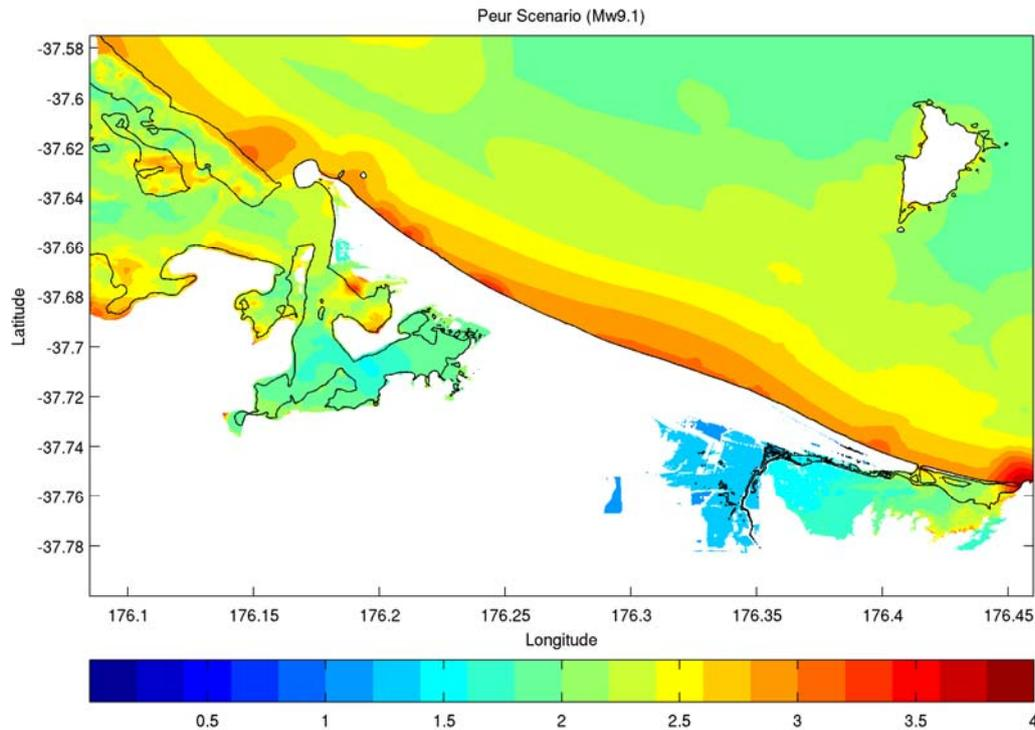
Figure 2.2 Maximum tsunami amplitude for the Peru ( $M_w$  9.1) fault rupture scenario along the Bay of Plenty coastline. The maximum tsunami wave ranges from 2.5m to 3.5m above MHWS. The shaded colour represents the maximum tsunami height above MHWS. Scale bar is in metres
