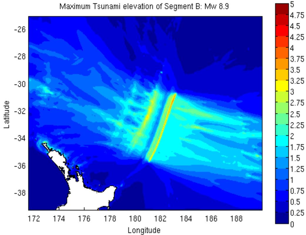
Figure A2.5 The maximum tsunami elevation above MHWS from the Central Kermadec Scenario. The colour scale shows the maximum tsunami elevation above MHWS. Scale bar unit is in metres.
