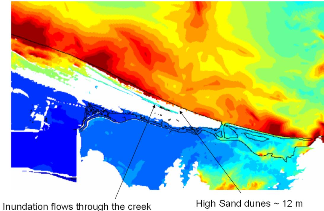
Figure A2.19 The maximum tsunami elevation above MHWS involving the Kermadec – Hikurangi Scenario for Te Tumu. The tsunami flows through the creek at the back of sand dunes at the Te Tumu as the sand dunes are high enough to prevent the tsunami inundating this area. Scale bar unit is in metres.
