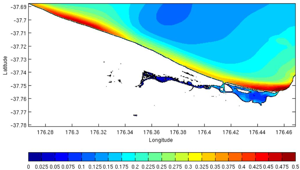
Figure A3.6 The maximum tsunami elevation varies from 0.2m – 0.5m above MHWS for the Volkner Fault along the Papamoa – Te Tumu coastline. The colour scale shows the maximum tsunami elevation above MHWS. Scale bar unit is in metres.
