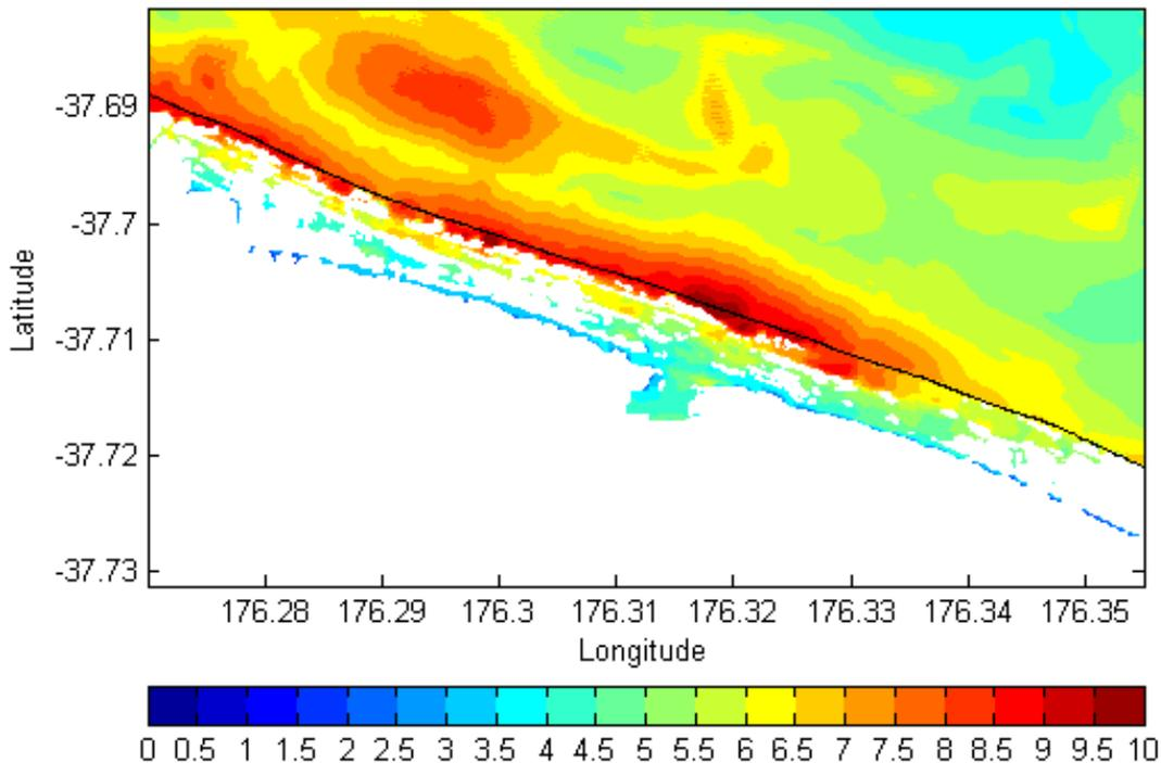
Figure A2.15 The maximum tsunami elevation above MHWS resulting from the whole Kermadec scenario for the Papamoa coastline towards Te Tumu. The tsunami overtops the sand dunes and inundates further inland through gravitational flows. The inundation follows the local terrain conditions such as the low-lying areas between the sand ridges. Scale bar unit is in metres.
