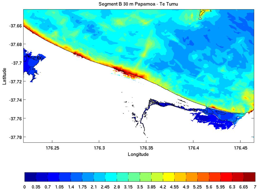
Figure 2.11 For the variation of the Central Kermadec Scenario, the detailed inundation modelling identifies localised inundation occurring along the Papamoa and Te Tumu coastlines. The tsunami from this event scenario is not capable of overtopping most of the sand dunes at Te Tumu. Localised inundation occurs at the low-lying area behind the Maketu Estuary. The colour scale shows the maximum tsunami elevation above MHWS. Scale bar unit is in metres.
