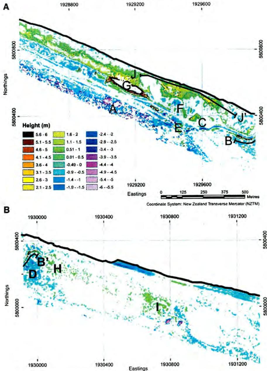
**Fig. 9.** Difference in vertical height between the 2000 and 2006 LIDAR data for (A) an area including the Awatarariki Stream and (B) an area to the east including the Matata Lagoon (locations shown in Fig. 2). Contours are at 1-m intervals. Lettered areas are referred to in the main text. Classification of heights around the mean has resulted in high values assigned no colour, as at area G. In this location, the maximum height is 11 m.
