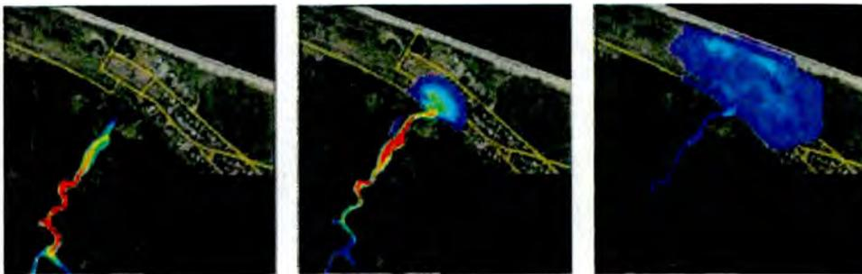
Figure 3. Output from the back analysis showing a large surge descending the Awatarariki Stream, emerging onto the fanhead and finally spreading across the coastal strip and western Matata. Colours indicate flow depths.
