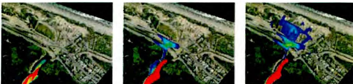
Figure 6. RAMMS output showing the predicted performance of the proposed barrier, dyke and raised building platforms. Colours indicate flow depths.
