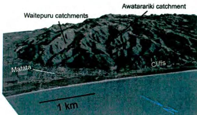
Fig. 3. The 3D perspective of the Awatarariki and Waitepuru catchments created using a 5-m DEM from LINZ 1:50,000 contours, and spot heights. The position of Matata and the coastal corridor seaward of the palaeo-cliffs are indicated.
