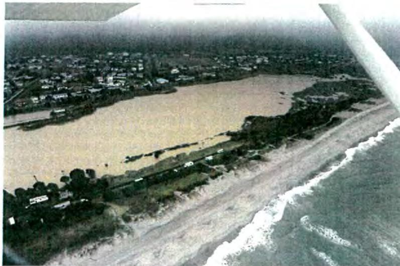
**Fig. 6.** Oblique aerial photograph (courtesy Whakatane Beacon, taken 18 May 2005), looking southwest, showing debris entering the western portion of the Matata lagoon, and associated silt-laden waters. Much of the fine sediment was not confined to the fan from the Awatarariki Stream, but was carried into the lagoon.
