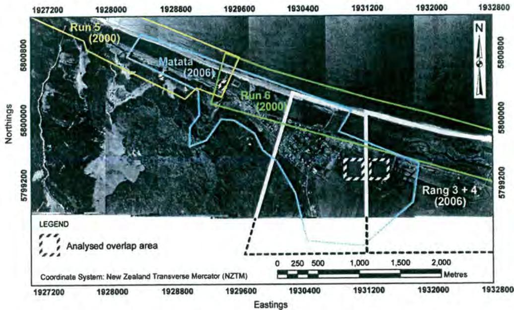
Fig. 7. Location of LIDAR data files—Run 5, Run 6, Matata, Rang 3 and Rang 4. Aerial photographs for context were flown in March 1987 by New Zealand Aerial Mapping Ltd. Areas of overlap used for analysis in producing the integrated pre-debris flow (2000) and post-debris flow (2006) topography are indicated.
