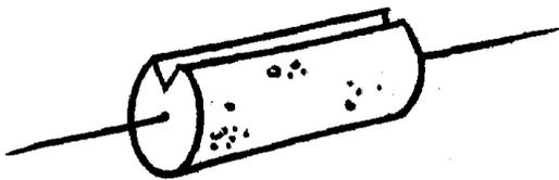
Push the wire carefully through the middle of the cork from end to end.
