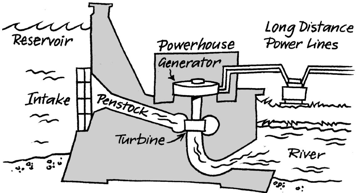
Hydro electric power plants use the power of falling water to turn the turbines that help generate electricity.
