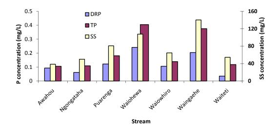
Figure 1. Mean concentrations for dissolved reactive P (DRP), total P (TP) and suspended sediment (SS) in 1993-94 for streams draining into Lake Rotorua (J. McIntosh, pers. comm.).
