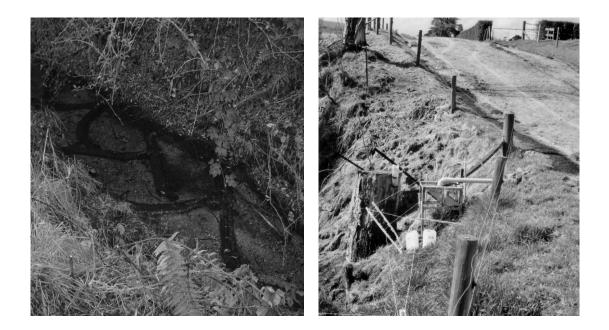
**Figure 5**. Picture showing the P socks installed on the bed of the Mangakino stream (left) and one half of the race with altered steel melter slag and tipping bucket installed (right). Note the Mangakino stream tributary flows through a culvert located below the tipping bucket.
