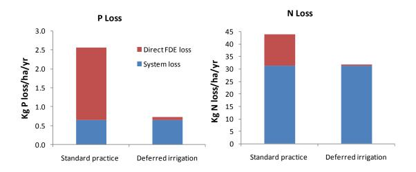
**Figure 3**. Comparison of FDE and system N and P loss from a single poorly timed application of FDE under "standard practice" and under deferred irrigation.
