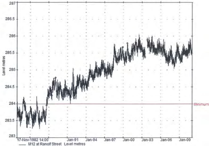
Figure 3: Long term water level (pressure) monitoring for monitoring bore M12. See Figure 1 for location.
