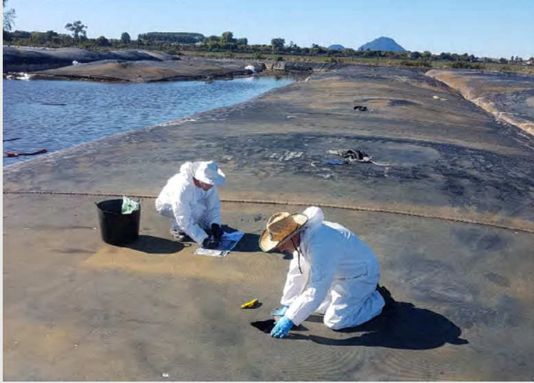
Photograph 7: Bioremediation team sampling within the Geobags at CS1.
