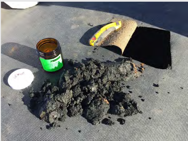
Photograph 6: Bioremediation team sampling within the Geobags at CS1. This core shows exclusively target material in the Geobag at this location.
