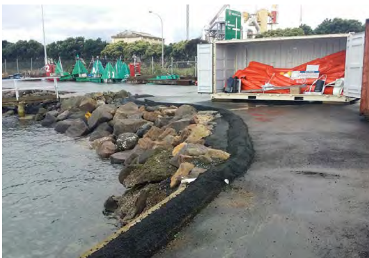
Butters Landing - Spill Equipment Container opened showing booms and equipment ready to be deployed
