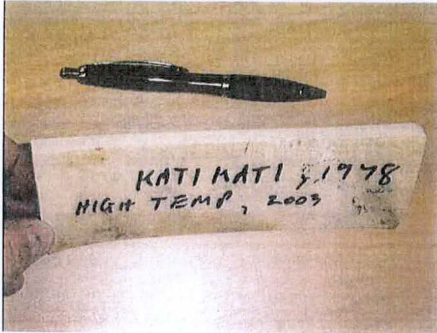
Plate 3.1: Pipeline sample subjected to high temperature stress relief testing
