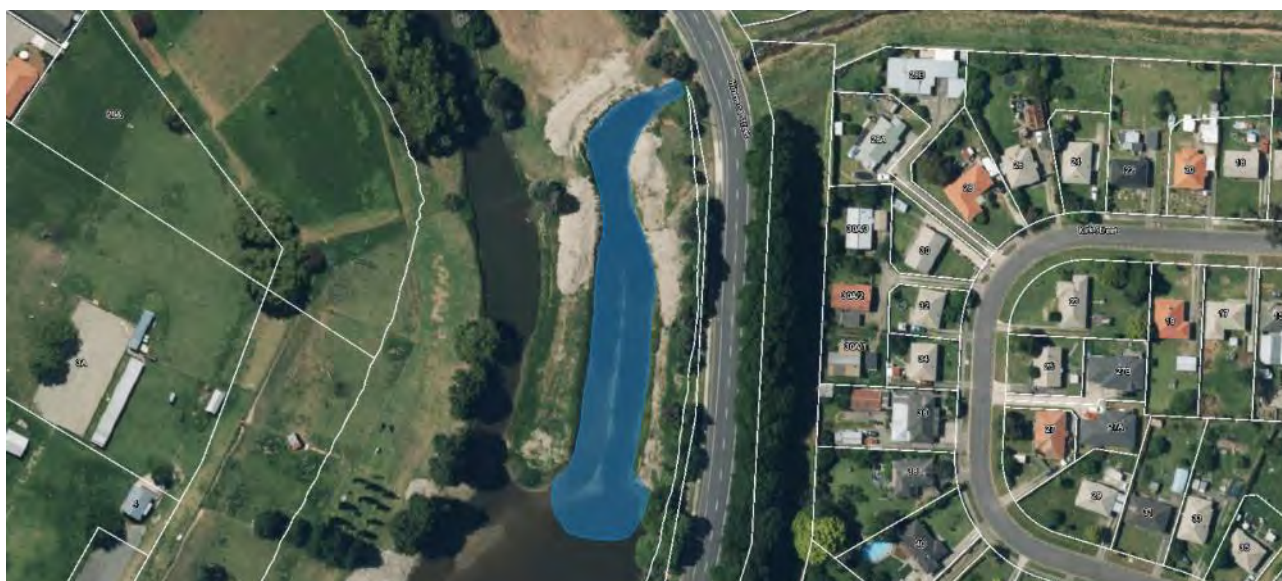
Figure 10. Awatapu delta (blue area) – used to managed fine sediment deposition from the Stream
