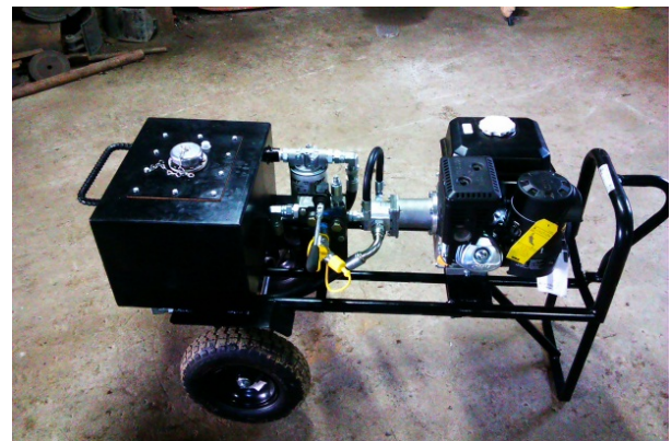
Figure 3.22 Hydraulic pack used to operate screw operated gates under hydraulic load.
