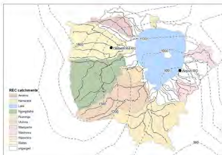
Figure 1: The spatial distribution of rainfall at Rotorua. Contour labels denote the rainfall scaling factor (RF multiplied by 1000) which is multiplied by the annual reference rainfall. Reference rainfall is the average at the Dalbeth Rd RG and Airport RG sites (solid circles). The outer catchment boundary shown is the surface catchment boundary derived using the REC which differs slightly from the surface catchment boundary used in this study (Lake_Rotorua_SC_1_2000_7_Mar_2014).
