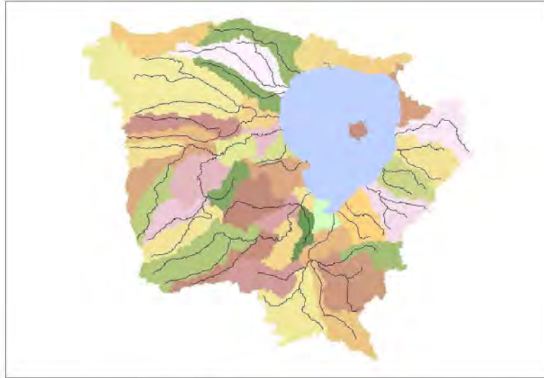
Figure 10: Surface sub-catchments. The catchments are those labelled CAT_70 in Rutherford et al. (2008) extended out to, or clipped by, the boundary GW_1_2000_16_Mar_2014_max1. Also shown are the main streams.
