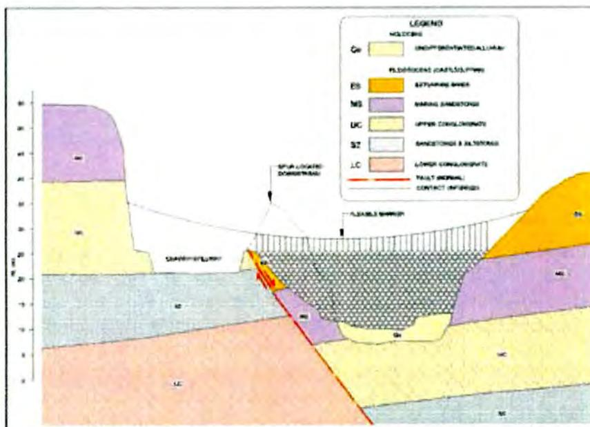
Figure 5. Section through the barrier location.
