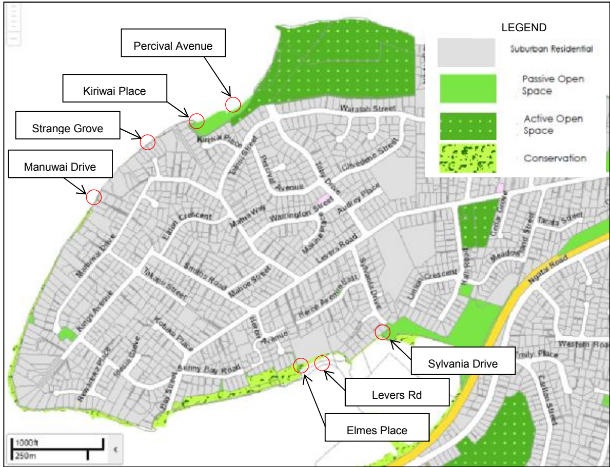
Figure 3-1: TCP Zoning and Potential Outfall locations
