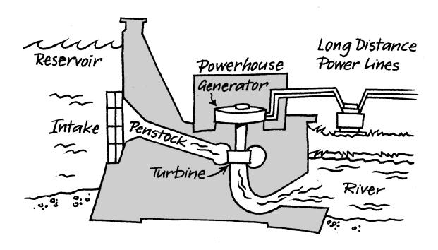
Hydro electric power plants use the power of falling water to turn the turbines that help generate electricity.
