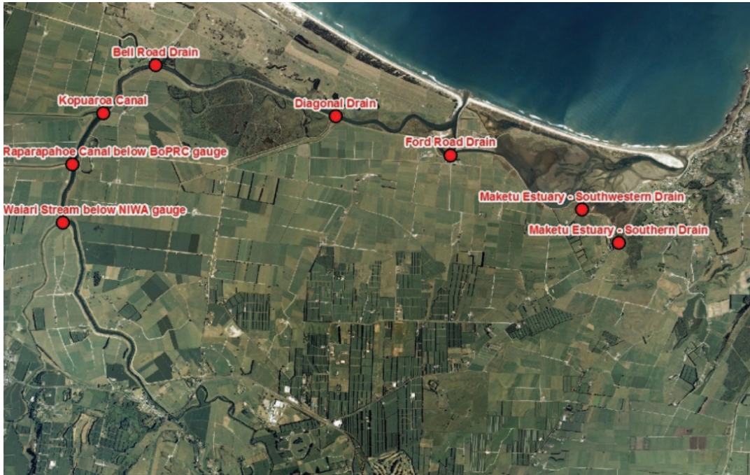
Figure 3-21 Predicted significant inflow locations into the estuary and river for the flood event that occurred over 17 th to 24 th April 2013.
