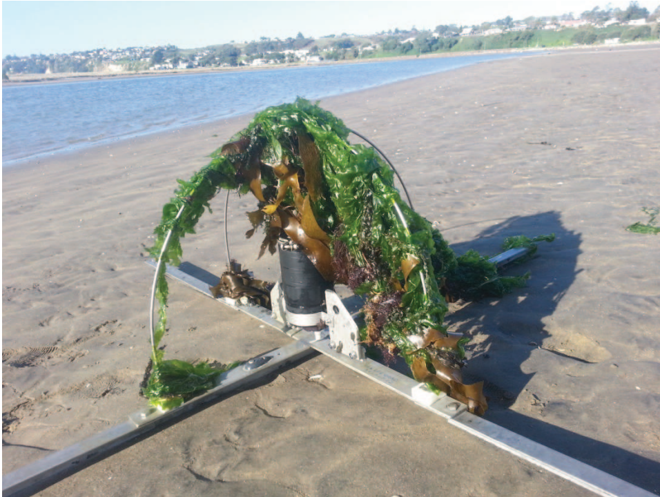
Figure 3-8 Fouling of current meter by Ulva. Instrument was deployed in vicinity of estuary entrance (see Figure 3-6).
