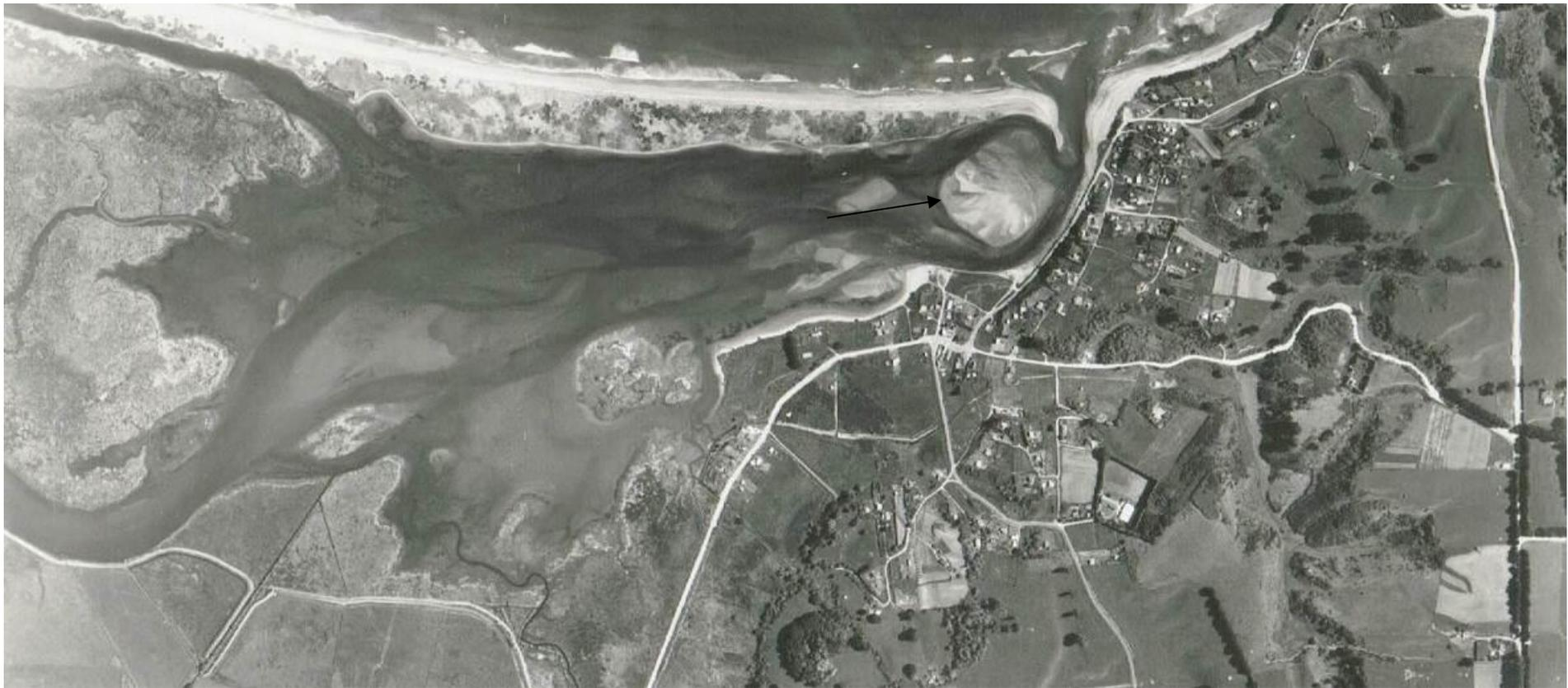
Figure 3: Aerial photograph of estuary dating from November 1959, shortly after diversion showing the enlarged flood tide delta (arrowed). See text for further discussion
