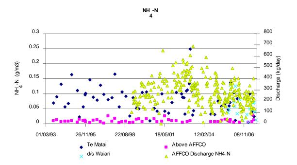
Figure 2.2.8 NH<sub>4</sub>-N concentrations at Te Matai and Above AFFCO and the AFFCO discharge load of NH<sub>4</sub>-N to the Kaituna River.
