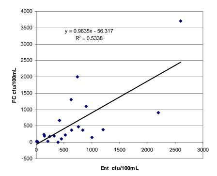
*Figure 2.6.2* Correlation between enterococci and faecal coliforms from the Ohope WWTP post maturation pond, 2003-2008 (data over 5000 cfu/100 mL omitted, one outlier omitted).
