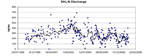
Figure 2.2.10 NH4-N discharge load from AFFCO treatment ponds, data and six month moving mean.
