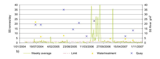
Figure 2.5.1 a) five week moving average of SS discharge from CHH Board Mill to the Whakatane River; b) weekly moving average of daily SS discharge load to river, and SS concentrations at two river sites.
