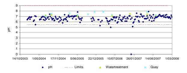
*Figure 2.5.2* Weekly pH results of CHH Board Mill discharge to the river and river pH results above and below discharge.
