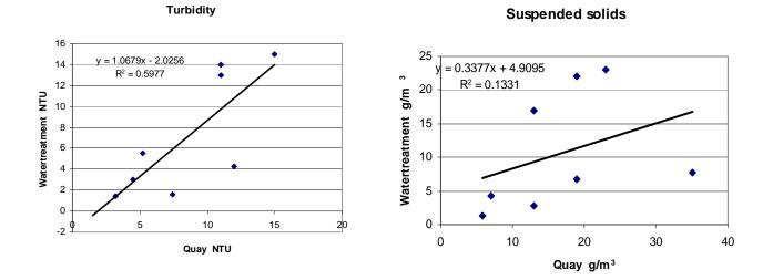
Figure 2.5.7 Correlation of turbidity and SS between the Quay Street and Water Treatment sites, 2002 to 2007 (one outlier removed).
