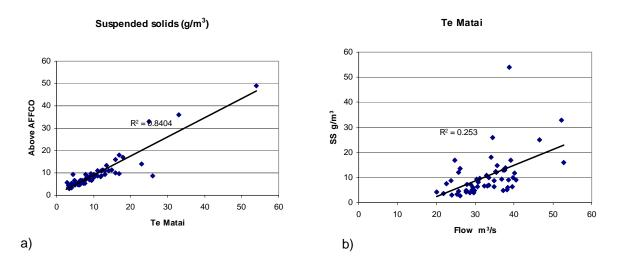
Figure 2.2.3 Correlation of SS data at above AFFCO and Te Matai (a); Flow vs SS at Te Matai (b).
