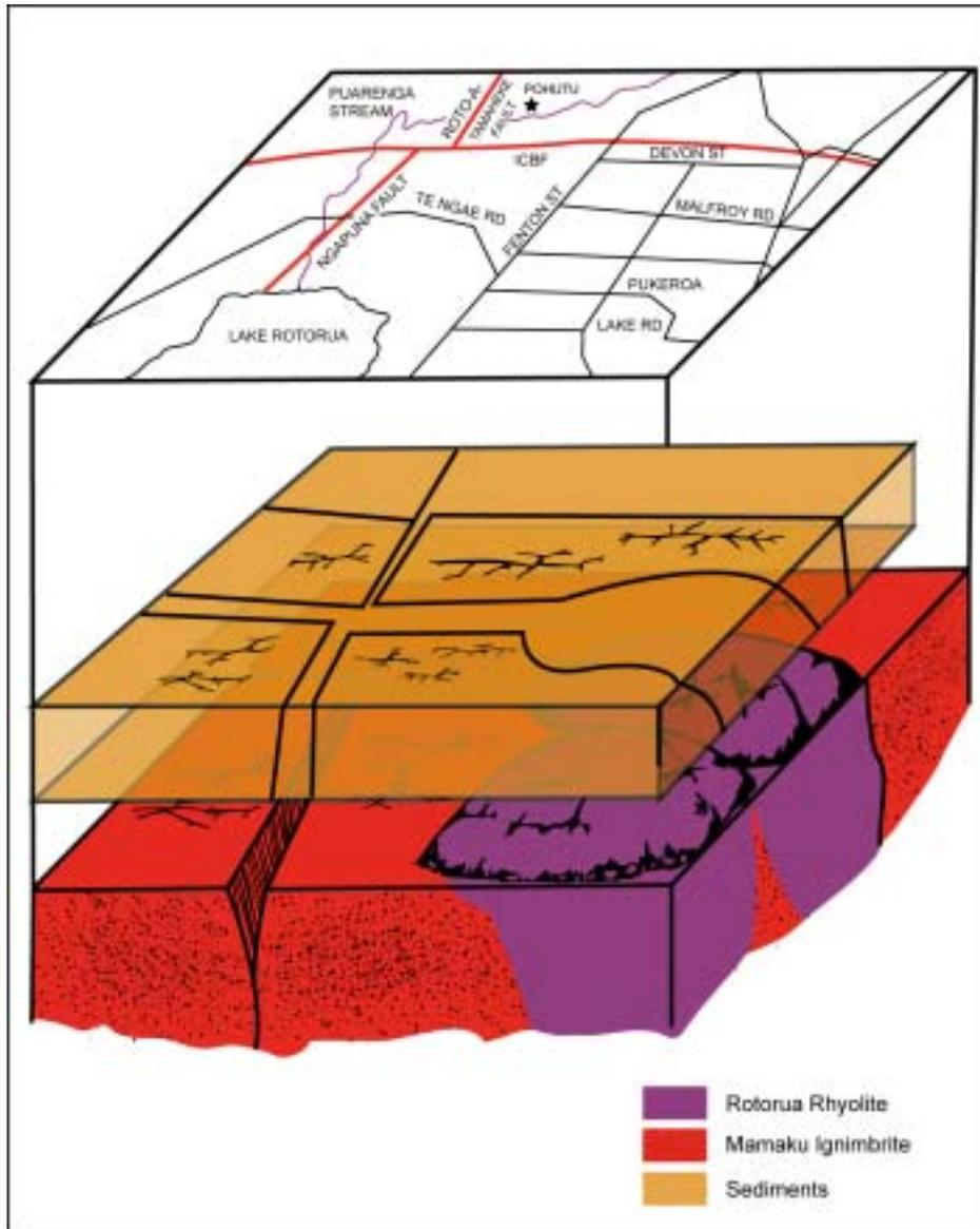
Figure 2.2 Block diagram showing the major geological and structural features of the field (after Drew 1985)
