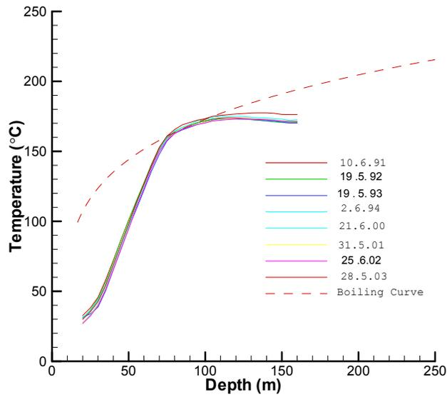
Figure 3.19 Temperature profiles for M17 (from Kissling, 2005)
