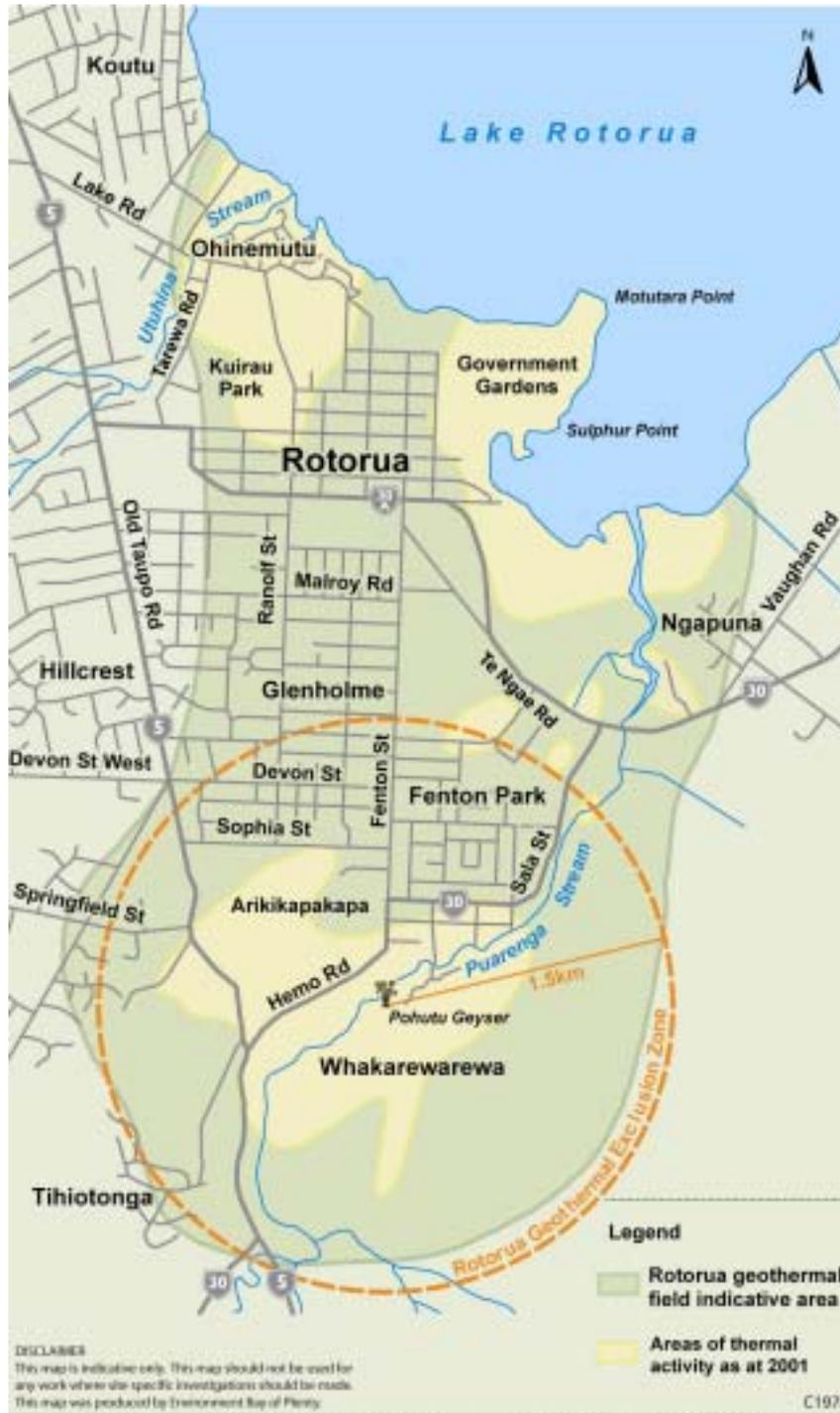
Figure 1.1 Extent of the Rotorua geothermal field as defined by the electrical resistivity surveys, and areas of surface geothermal activity. Also shown is the 1.5 km Rotorua Geothermal Exclusion zone.
