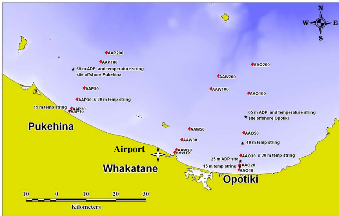
Figure 2.3 Temperature string, ADP deployment and transect sites within the Bay of Plenty. Also shown is the location of the Whakatane Airport.
