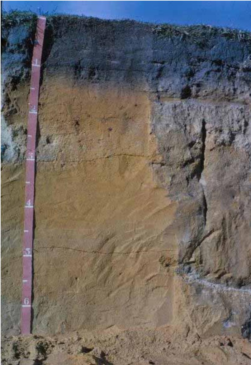
**Manawahe loamy sand** (Note deep topsoil formed from fine Tarawera Tephra and the buried topsoil of Kaharoa Tephra, scale in ft)
