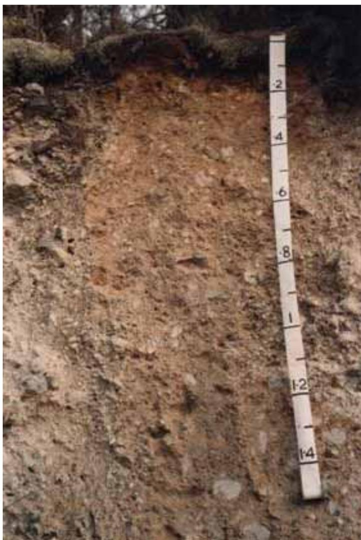
**Kaingaroa gravelly sand** (Note very shallow topsoil and B horizon, and the coarse poorly sorted angular pumice throughout the soil profile, scale in m)
