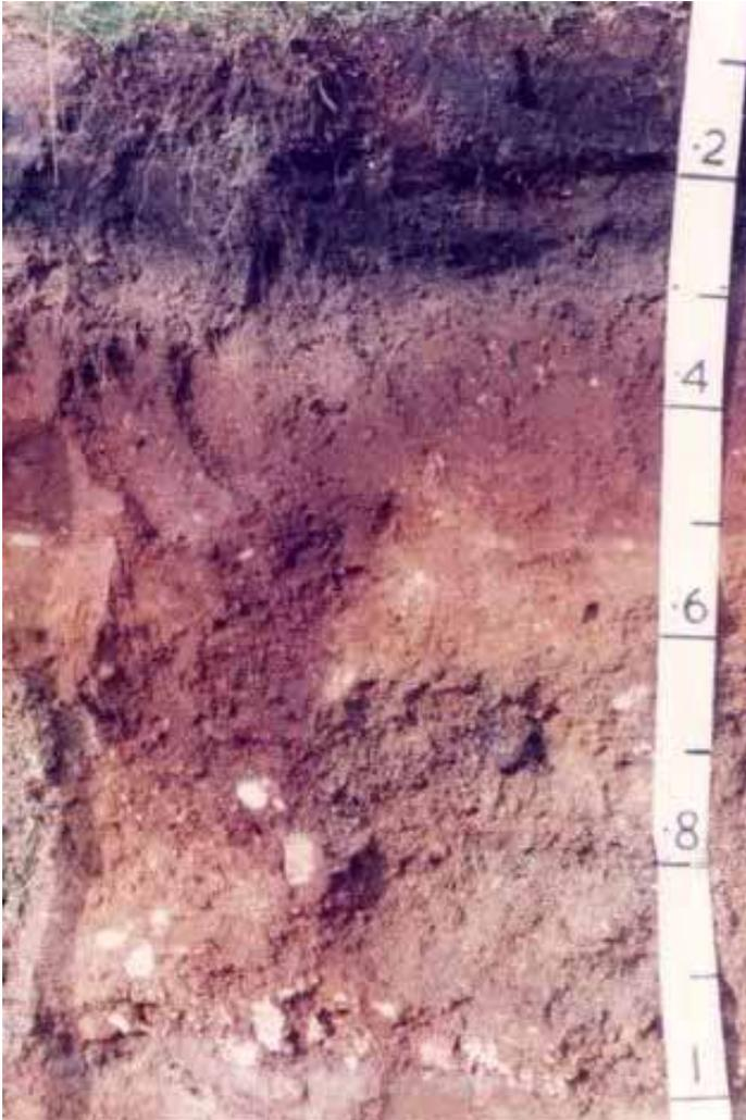
**Tihoi sandy loam** (Note pale horizon below black topsoil and red iron staining in subsoil, scale in m)
