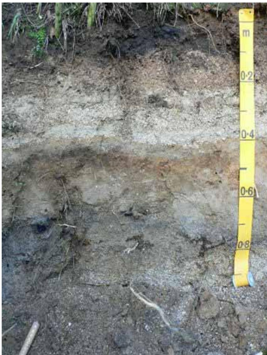
**Te Rere sand** (Note thick band of white Kaharoa lapilli at the surface)
