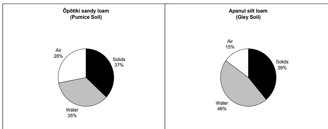
*Figure 5.2 Volume composition of a well-drained soil (Ōpōtiki sandy loam) and a poorly-drained soil (Apanui silt loam). Both soil types have almost equal pore space, but the volume occupied by air is much less in the poorly-drained soil because its pore space is largely occupied by water.*
