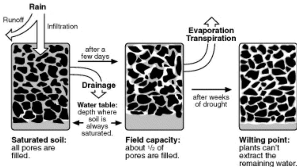
Figure 5.1 Soil water retention and depletion process illustrating the concepts of saturation, field capacity and wilting point. Available water-holding capacity is the amount of water retained between field capacity and wilting point (Source: University of Minnesota 2000).
