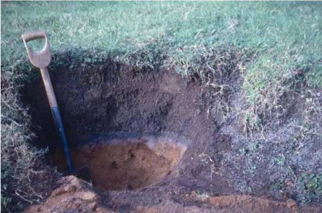
**Tarawera gravel** (Note thick coarse Tarawera Tephra and buried topsoil of Kaharoa Tephra)
