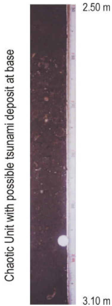
Figure 15: Waihi Beach – Detail of Core WAI 1 from approx. 2.50-3.10 m showing chaotic layer and possible tsunami deposit (unclear in photo) – refer to Figure 14 for details.
