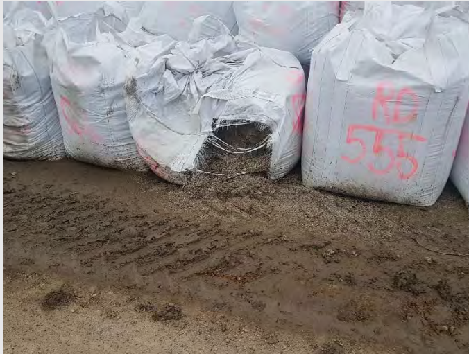
Photograph 20: Damaged bulk bag spilling oversized sediment.
