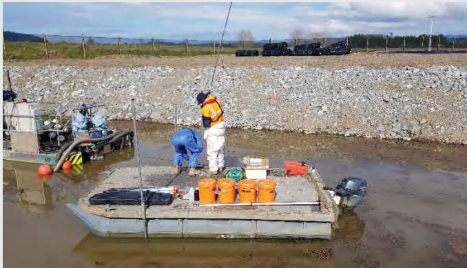
Photograph 14: GAL undertaking sediment validation within the Kopeopeo/Orini Pump Station intake channel.
