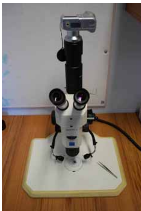
Figure 6.1 Zeiss Stemi V2 stereo microscope setup with digital camera
