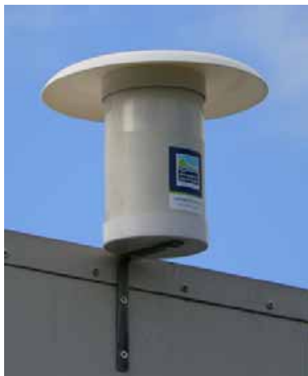
Figure 8.4 Directional dust sampler (note: adhesive film is positioned within the top third of the sampler)
