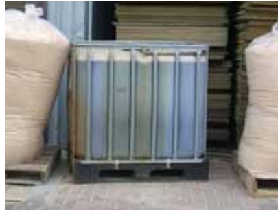
waste oil is left on a hard stand for collection. There is no protection from spills that may occur during storage or loading. Products should be stored and loaded in an area where spills will be contained.
