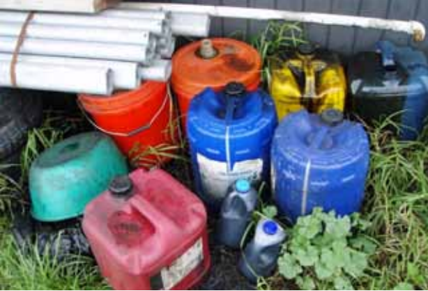
(Above) poor storage of waste oil allowing soil contamination. These containers should be stored in a covered and bunded area.
