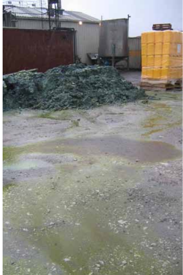
(Above) an uncovered stockpile causes water and soil contamination during rain. This stockpile should be covered or indoors.
