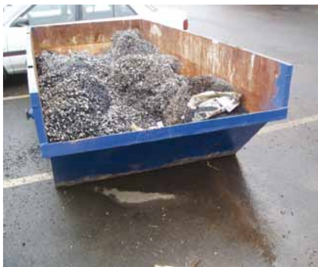
(Above) scrap metal filings are stored in an open skip. Transferring of waste has led to spill around the skip which will be washed to stormwater when it rains. Positioning of skips is important to prevent tracking and spreading of waste from the source.
