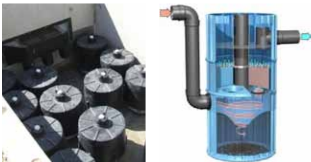
(Above) end of line treatment devices, such as, using filter pods or hydrodynamic separation can be used to treat run-off. These need to be appropriate to the volume and type of run-off.
