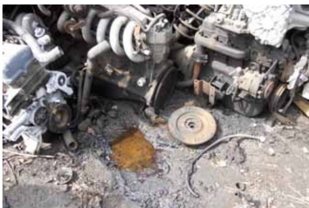
(Above) poor storage of engines allowing soil contamination.
