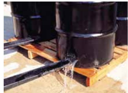
drums punctured by a forklift. Loading areas should be isolated or have a spill containment area where leaking drums can be placed quickly.
