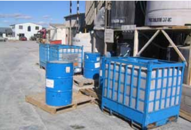
(Above) poor storage of IBC's and drums without any form of spill containment.
