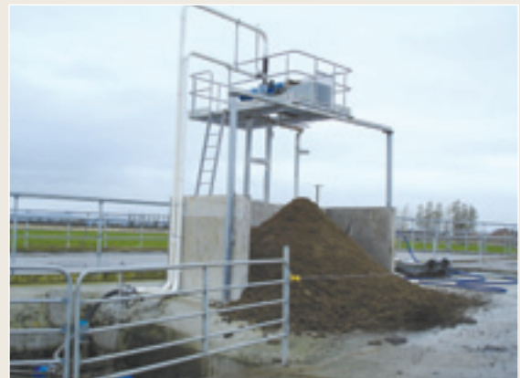
Solids separation machines provide easily handled solid and liquid products.
