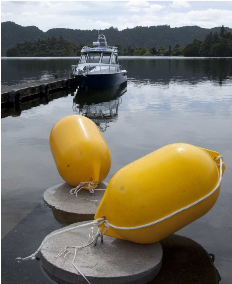
Picture 1 Main anchoring weights and floats prior to deployment
