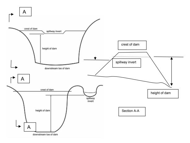
Figure 4.1 Cross-section of a typical small dam defining measurement of the dam water retention height (Source: Regional Water and Land Plan, Bay of Plenty Regional Council, 2008).
