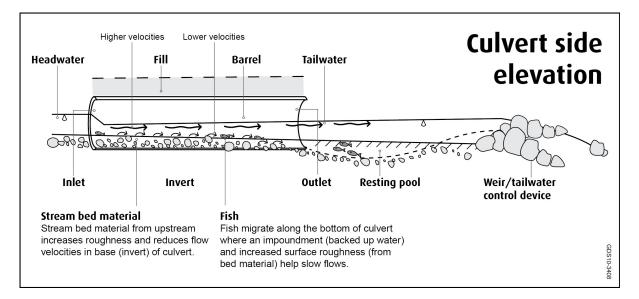
Figure 7.3 Culvert details suitable for fish passage
