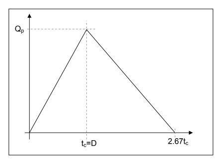
Figure 5.1 Simple hydrograph for storm flow
