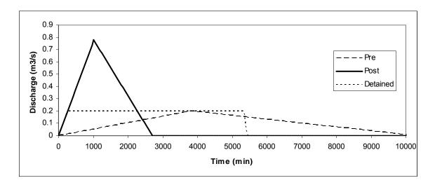
Figure 5.2 Sample Pre-, Post- and Detained hydrographs
