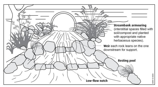
A succession of weirs helps raise the water level so it creates an impoundment through the culvert.
