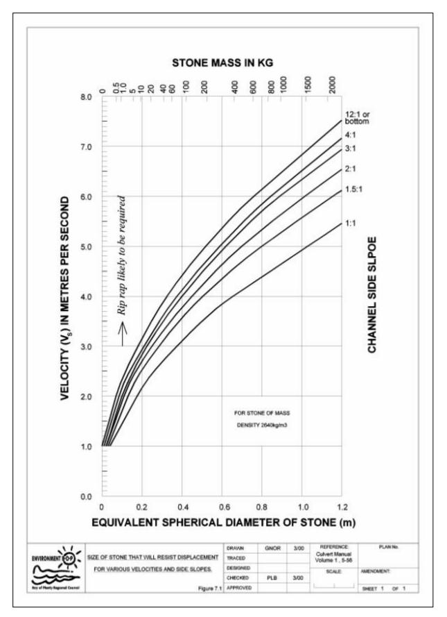
Figure 7.1 Rip-rap sizing diagram to determine d50
