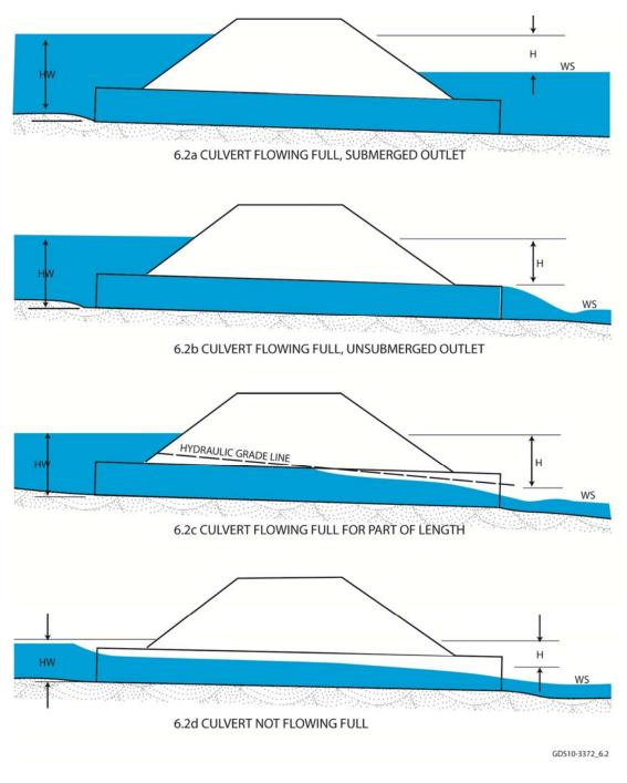
Figure 6.2 Flow profiles for culverts under outlet control
