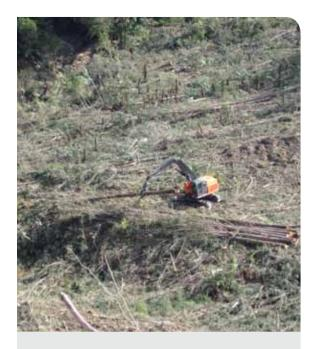
Shovel logging to stack logs ready for the hauler leaves slash and logging residue relatively undisturbed, and protects the soil surface before replanting
